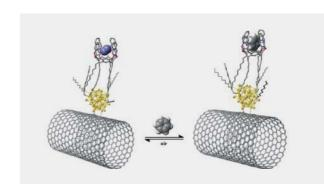
Patent WO2016079356 > resistive sensor for detecting benzene gas and method for the production thereof
