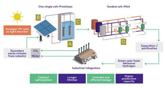
"sustainable processes to produce hydrogen and methanol as energy vectors using only sunlight as an energy source and wastewater and CO2 as feedstocks"
